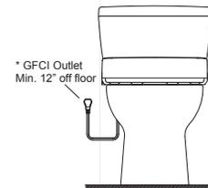
\* The 3-prong cord on the Washlet is on the left side and is 3' long. The GFCI outlet needs to have 120V, 10amps.
