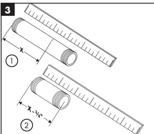
Remove the test nipple and measure it to the mark ("X").
