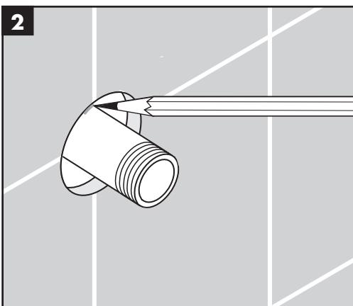
When the finished wall is complete, mark the test nipple at the wall surface.
