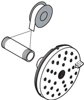
Wrap the threads on both ends of the nipple with Teflon tape.
