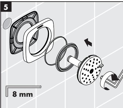
Hold the sealing ring against the wall.
