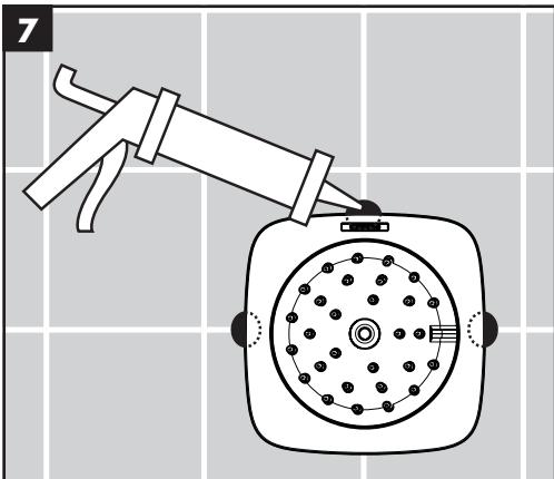
Place a small amount of waterproof sealant at the top and side grout joints.
