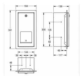
Double toilet roll holder with spindle system for recessed mounting, stainless steel, surface satin finished, material thickness 22 gauge folded front cover, cylinder lock with Franke standard key, for 2 rolls with max  $\emptyset$  120 mm (4 3/4"). Second roll will be released after consumption of first roll, reserve roll not visible, including stainless steel screws and dowels.
